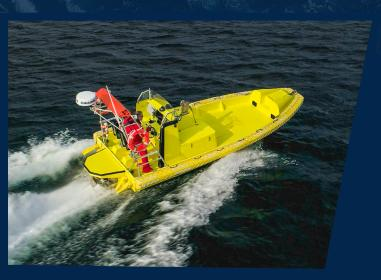
The fender is constructed of closed cell polyethylene foam. Not deflating with solid core that cannot lose buoyancy or absorb water. Damage is strictly cosmetic keeping crew safe. For further protection the foam fender is covered with a heavy-duty tarpaulin, with a netting attached. This allows a person in the water to grab onto the fender, for easy recovery.
